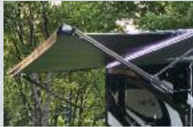
POWER AWNING WITH LED STRIP Extend and retract your awning with the push of a button. Both arms are adjustable to get just the right angle.
